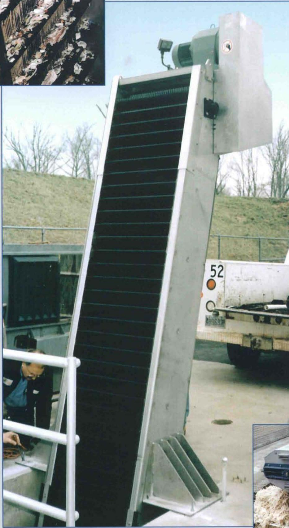
The CleanFlo™ is a continuous belt-type finger screen designed to remove debris from water and wastewater. With capacities to 100 MGD and discharge heights exceeding 50 feet, CleanFlo™ screens can handle the most demanding applications. These units are designed and built to customer specifications and are easily customized for particular needs. Retrofit installations involving deep or wide channels present no difficulty for the CleanFlo™.
