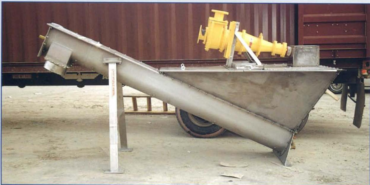
When Gritt Mitt is equipped with an optional cyclone, it will remove 95% of 150 mesh grit and can accommodate much higher flows. The cyclone uses hydraulic forces for separation and has no moving parts for cleaner operation and low maintenance without fouling.
